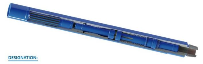
Reciprocator is designed for releasing stuck downhole toll by impacts directed up and down in turns together with static axial load and torque. Reciprocator is used as a bottom section of impact assembly together with hydraulic jars JGB or JGR.
